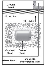
stone. To minimize stress on the tank and connection in the event of shifting of the sand surrounding the tank, we recommend the use of a swing joint connection (see diagram). Make sure to completely backfill the hole with sand and compact to prevent tank settling. Permanently mark and identify the location of the tank.
